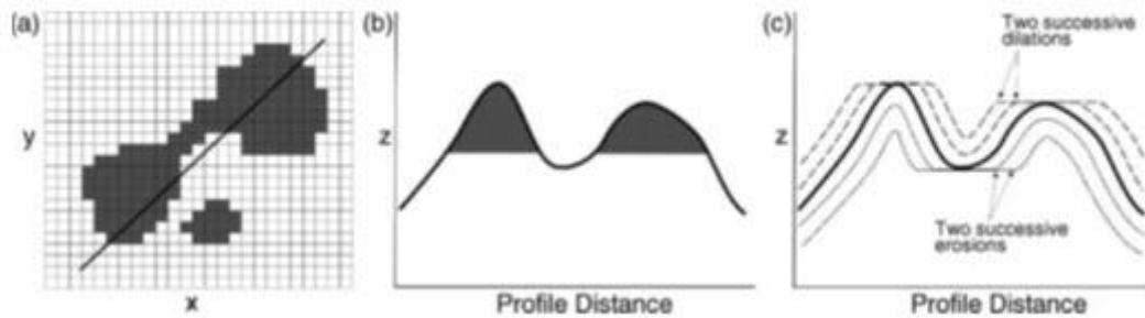
Fig. 1.6 (a) The original input image with the position of a profile line marked; (b) the theoretical cross-sectional profile with the shaded area representing the geographical extent of the darker class along the line shown in (a); and (c) the effect on the profile of dilations and erosions of that surface.
